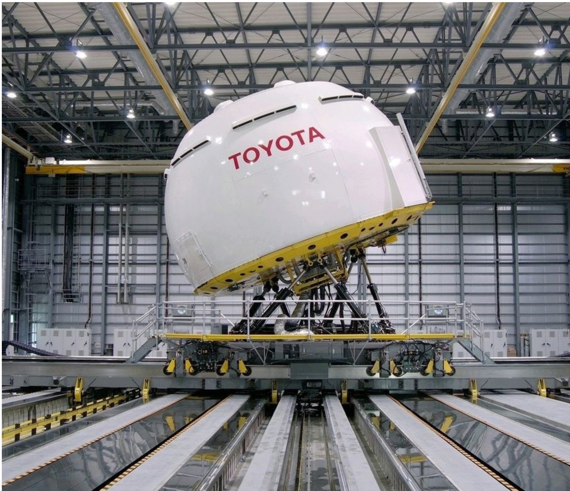
Driving simulator Toyota Higashifuji Technical Center
